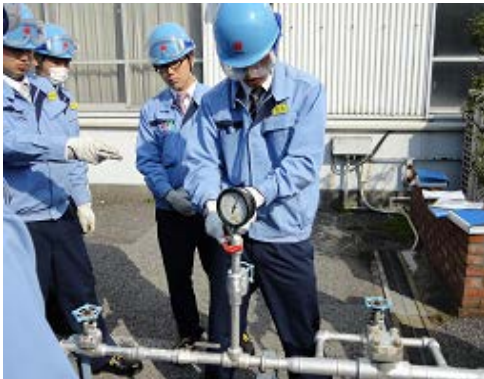
valve seat leakage
